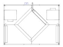
8 sizes for air volumes from 290m3/h to 4000 m3/h. Static cross-flow heat recovery unit with minimum efficiency 50%.
