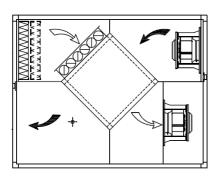
3 sizes for air volumes from 1500m3/h to 5500 m3/h. Static cross-flow heat recovery unit with 65% efficiency with by-pass. High efficiency directly-driven fans with brushless motor.
