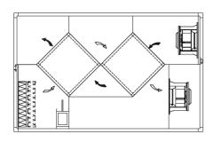
3 sizes for air volumes from 1000m3/h to 5000 m3/h. Static cross-flow heat recovery unit with minimum efficiency 90% with option for total air by-pass. High efficiency directly-driven fans with brushless motor. AISI 304 stainless steel drain pan. Filters class G4 on fresh air intake and exhaust side with option for compact bag filters class F7. Option for external installation and vertical execution. Accessories: heating coil, cooling coil, electric battery, control board.
